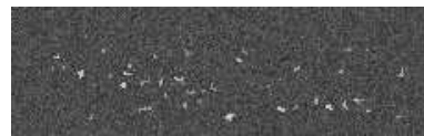
Figure 2: An artificial image ( \mu_b = 0.3, \sigma_b = 0.055, i = 1, \dots, 100, \mu_{\sigma_d} = 0.01, \sigma_{\sigma_d} = 0.002, \text{foreground/background ratio} = 0.015, \mu_{P_d} = 5, \sigma_{P_d} = 3 ).
